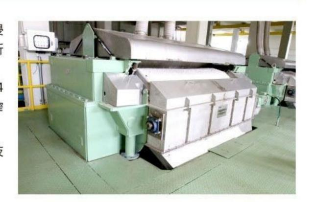
Introduction: AC press is one of the key equipments for the production of viscose staple fibers. Its function is to press the pulped alkali cellulose to remove excess water and finally achieve the composition for xanthating reaction. The working width of AC press produced by 1 900mm, 1800mm, 2400mm and so on. The corresponding capacity is 16 t/d, 33 t/d, 44 t/d, of which 2400mm working width of the machine is the largest width and the most productive AC press.
