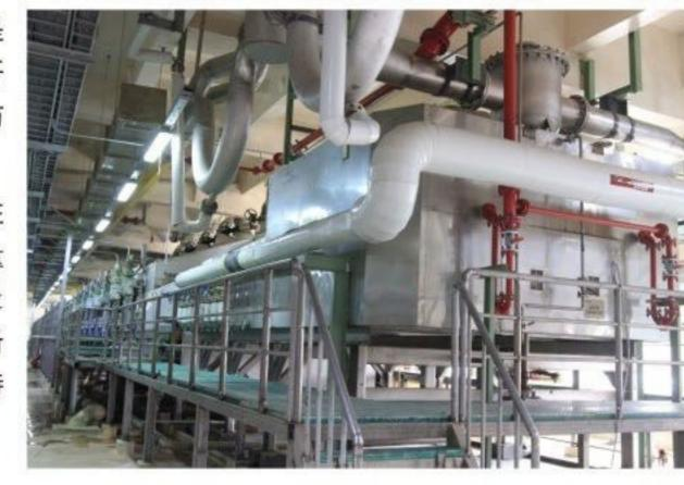
The After-Treatment Combination Machine is composed of trunklines, CS2 recovery trough and After-Treatment machine. Its function is to clean the cut-off fiber, remove the acid impurities that were contained in the fiber, bleach and grease the fiber. The fiber will have a certain degree of whiteness and good spinnability.
